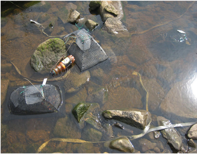
Figure 2. Stream bed set for shock treatment, with electrode tapes and test cages (6 mm plastic mesh, base 30 × 45 cm, with gravel and 15 signal crayfish).
