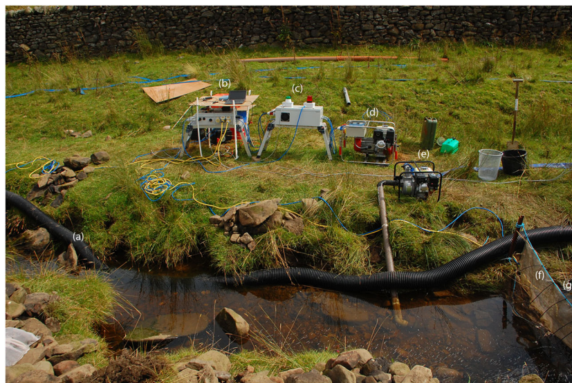
Figure 1. Equipment set-up for electric shock treatment of a stream: (a) flume pipe for flow bypass; (b) pulse unit and laptop computer for programming; (c) capacitor unit; (d) 5 kW generator; (e) pump for dewatering after treatment; (f) stop net; section under treatment.
